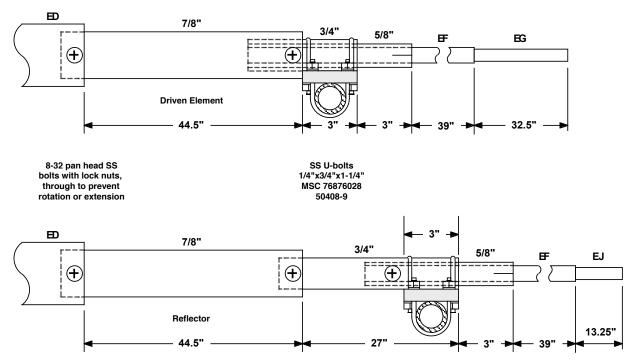
The element assemblies consist of the following sections, also shown in a different view below:
