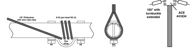
The guy cables are attached to the vertical strut through 5/16" turnbuckles to a clamp made from a "pipe repair clamp," ACE Hardware #41834, with 1/4" SS bolts and locknuts substituted.
