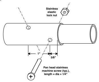
The tip sections EF can be secured with either hose clamps on the 5/8" extensions or cross-bolts. The exposed length of EF can be shortened by 3" (to 42") and the exposed length of EG and EJ can be extended by 3" to use cross-bolting, with no measurable effect on element tuning.
