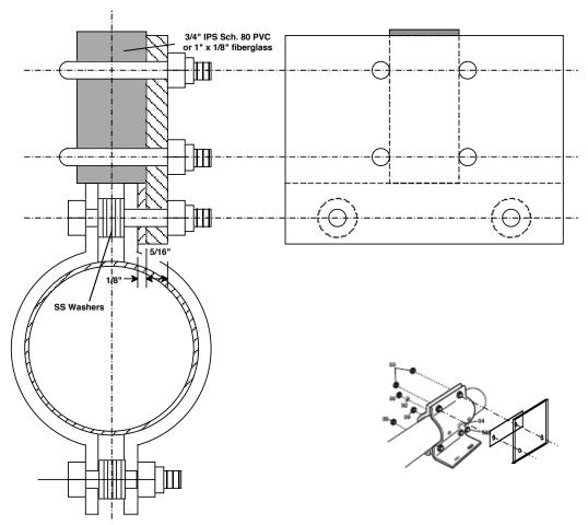
The element guy is 1/8" Phillystran, with 1/8" cable clamps (3 per end). The guy rope is wound one or more times around the element, so no thimbles are required. The location of the guy on the element is held by a stainless eyestrap or fairlead (Eyestrap - Narrow, 1-1/4"L x 3/8"W #8 holes West Marine #120667 RF498). The details of the attachment to the element with two stainless 8-32 through bolts, washers and lock nuts are shown here<sup>2</sup>:
