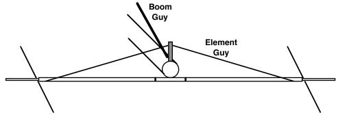
The vertical brace is a 36" length of 3/4" IPS Schedule 80 PVC pipe or conduit or 1" x 0.125" fiberglass tube, held in place by a bracket mounted to the side of the element-boom clamp #509:
