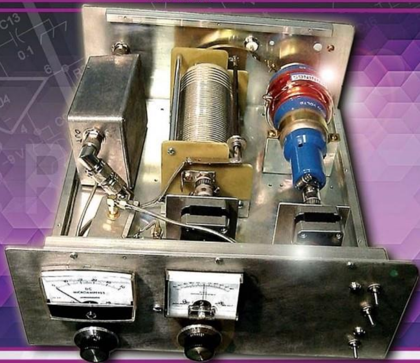
W8MQW L-network Matchbox uses a stepper-driven vacuum capacitor and a roller inductor.
