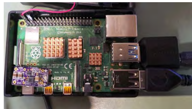
Raspberry Pi 4 with Switching Mode Power Supply for Grape Receiver and GNSS Disciplined Oscillator
